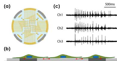
A planar grid of microelectrodes (a) interfaces with cultured neurons (b), modeling in vivo neural behavior in a dish. Electrodes detect changes in raw voltage (c) through recording of extracellular field potential.
