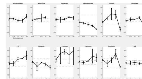
Burst strength, as discussed above, is also shown for all 12 compounds included in the HESI NeuTox pilot study. The "dashed" gray lines indicate the detection limits defined by the vehicle control replicates on each plate. 8 of the 9 proconvulsant compounds were detected for at least one concentration tested, with many displaying clear dose-dependent trends. Further work will focus on additional endpoints and the development of statistical models to detect proconvulsant compounds.
